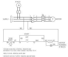
SEPARATE NO-VOLT SUPPLY - REMOVE LINK BETWEEN 1 ON C & 96 ON OL AND 5 ON C & A1. CONNECT SEPARATE SUPPLY TO 96 ON OL & A1.
